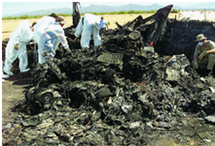
Figure 11. Compact Mishap Sites Can Present Challenges for Searching in Wreckage and Sketching the Scene.
